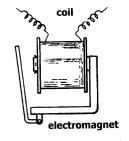
At least, to actuate this assembly, we put a coild around the core.
